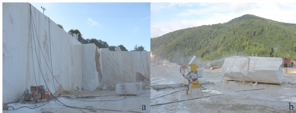
Fig. 5. Marble exploitation equipment in Dealu lui Ionel (Ionel Hill) Quarry (a. kerving machine and b. diamond wire saw machine)
