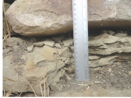
Fig. 3. Partial disintegration caused by severe delamination.
