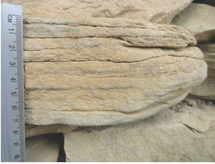
Fig. 2. Severe delamination along the bedding planes.
